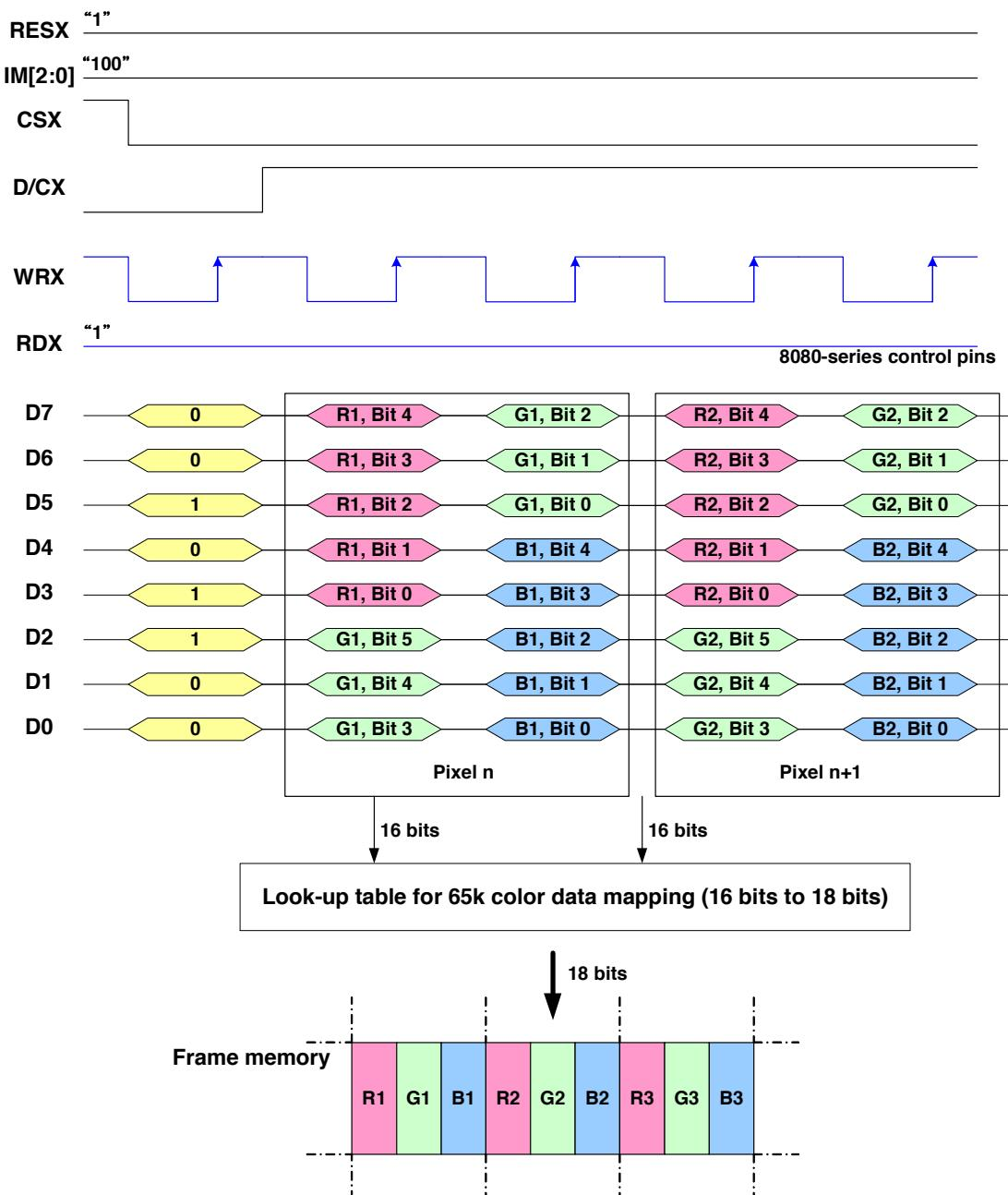
Note 1: The data order is as follows, MSB=D7, LSB=D0 and picture data is MSB=Bit 5, LSB=Bit 0 for Green and MSB=Bit 4, LSB=Bit 0 for Red and Blue data.
