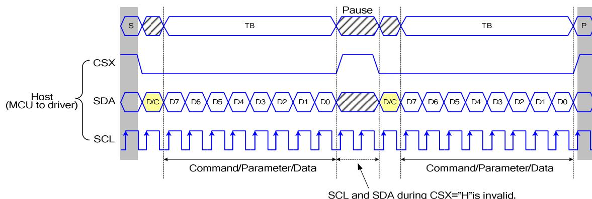
Figure 25 Serial Interface Pause Protocol (Pause by CSX)
