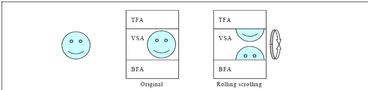
When Vertical Scrolling Definition Parameters (TFA+VSA+BFA) =162. In this case, ‘rolling’ scrolling is applied as shown below. All the memory contents will be used.
