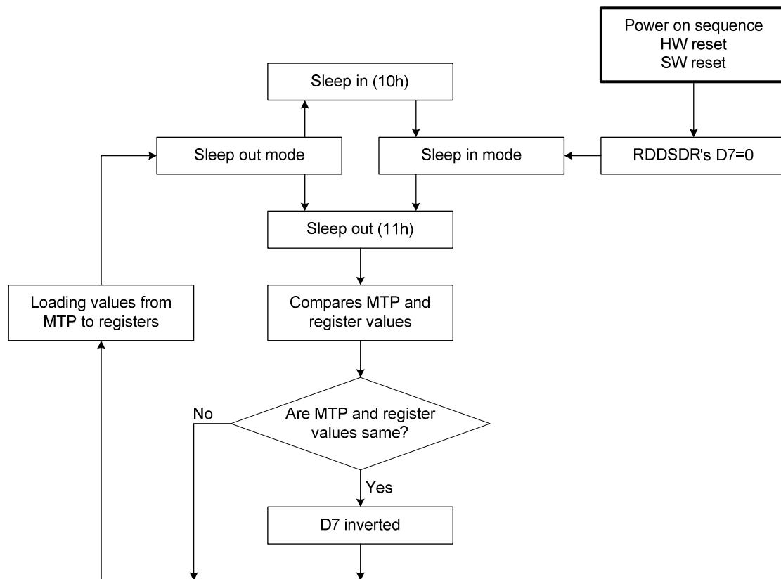
*Note: There is not compared and loaded register values, which can be changed by user (00h to AFh and DAh to DDh), by the display module.*
