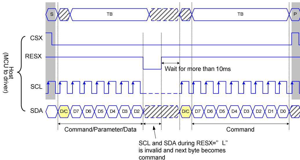
Figure 21 Serial Bus Protocol, Write Mode – Interrupted by RESX
