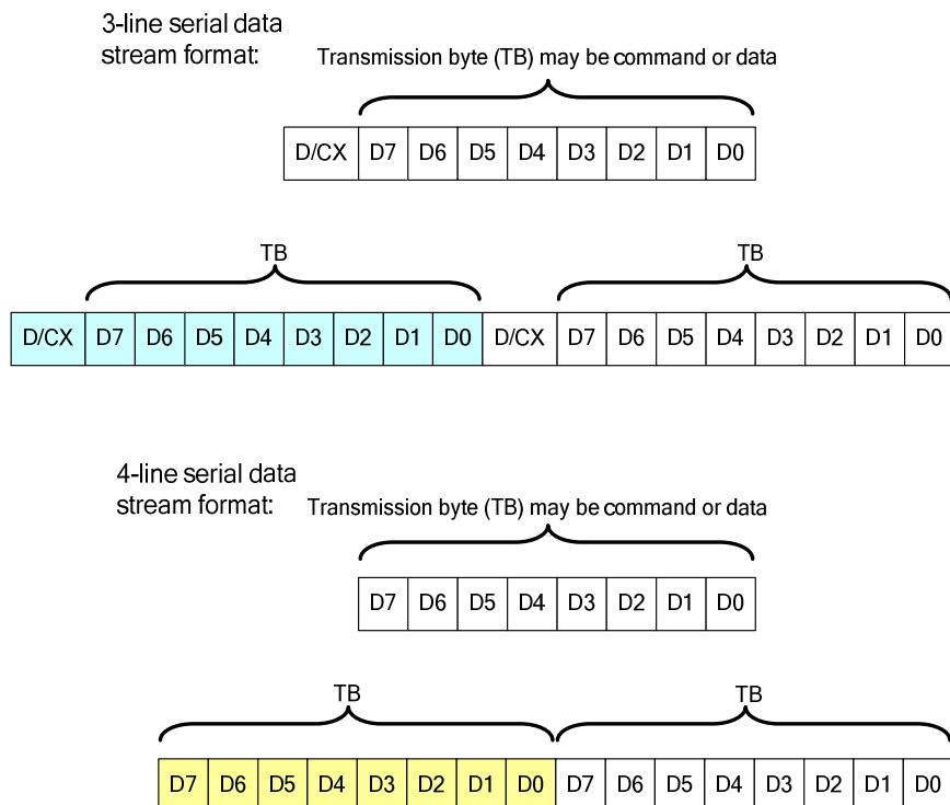
Figure 16 Serial Interface Data Stream Format
