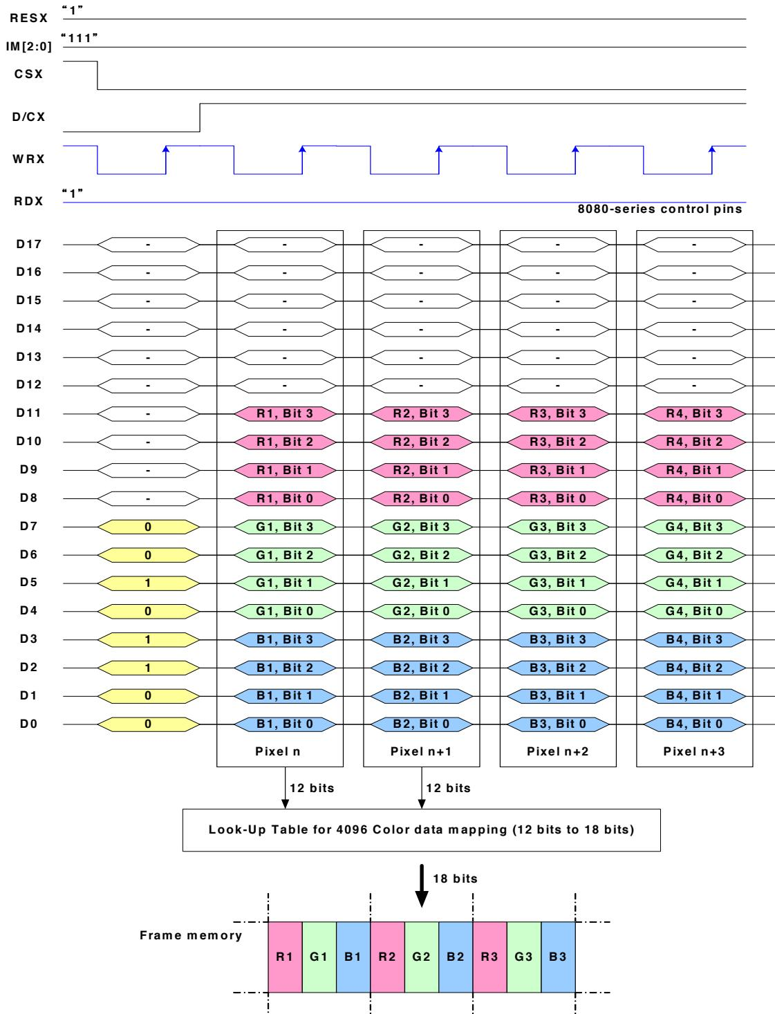
Note 1: The data order is as follows, MSB=D11, LSB=D0 and picture data is MSB=Bit 3, LSB=Bit 0 for Red, Green and Blue data.
