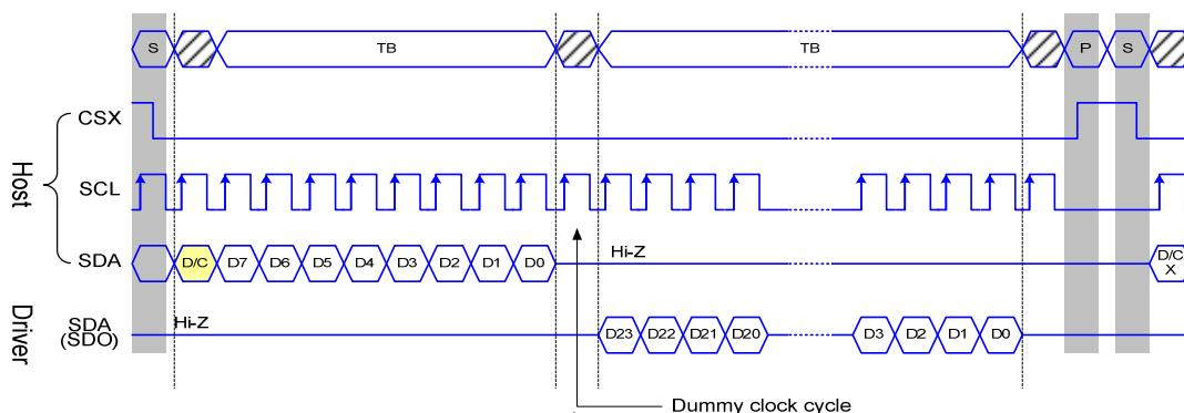
3-line Serial Protocol (for RDDST Command: 32-bit Read)
