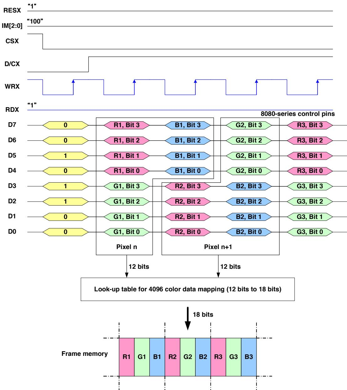
Note 1: The data order is as follows, MSB=D7, LSB=D0 and picture data is MSB=Bit 3, LSB=Bit 0 for Red, Green and Blue data.
