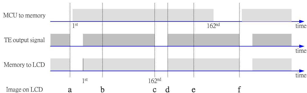
The MPU to Frame Memory write begins just after Panel Read has commenced i.e. after one horizontal sync pulse of the Tearing Effect Output Line. This allows time for the image to download behind the Panel Read pointer and finishing download during the subsequent Frame before the Read Pointer “catches” the MPU to Frame memory write position.
