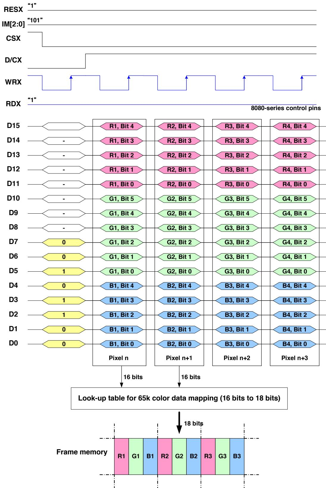
Note 1: The data order is as follows, MSB=D15, LSB=D0 and picture data is MSB=Bit 5, LSB=Bit 0 for Green, and MSB=Bit 4, LSB=Bit 0 for Red and Blue data.
