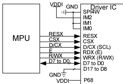
**13.3.6 6800-Series MCU Interface for 16-bit Data Bus (P68=1, IM2, IM1, IM0="101")****68 Serial MPU 16-Bit Bus**
