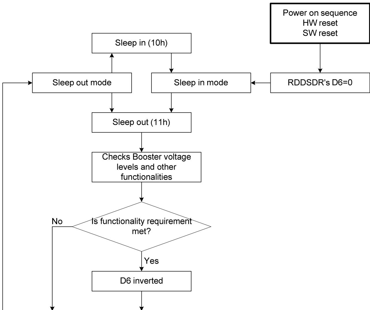
*Note: There is needed 120msec after Sleep Out -command, when there is changing from Sleep In -mode to Sleep Out -mode, before there is possible to check if functionality requirements are met and a value of RDDSDR's D6 is valid. Otherwise, there is 5msec delay for D6's value, when Sleep Out –command is sent in Sleep Out -mode.*
