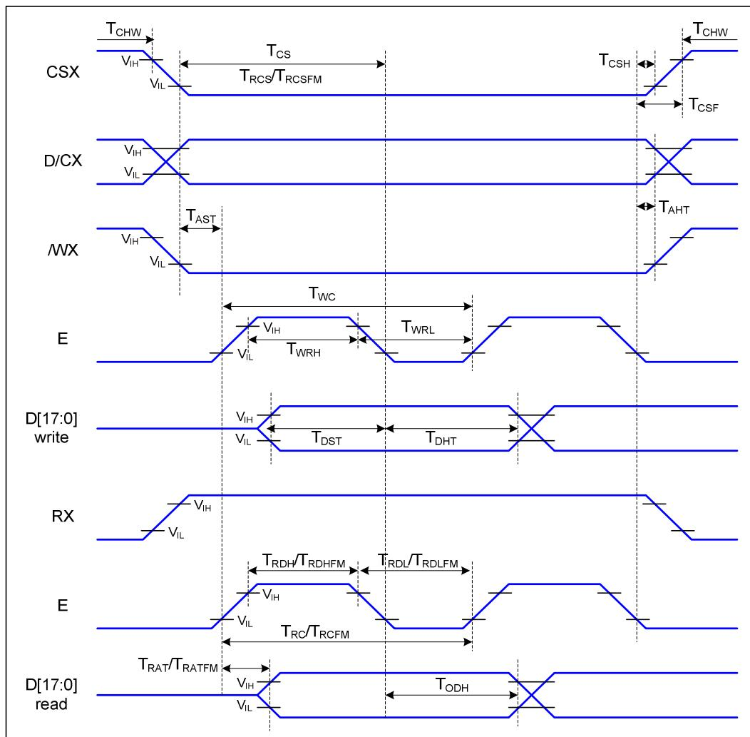
Figure 5 Parallel Interface Timing Characteristics (6800-Series MCU Interface)
