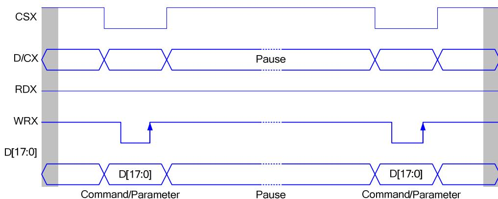
Figure 26 Parallel Bus Pause Protocol (Paused by CSX)
