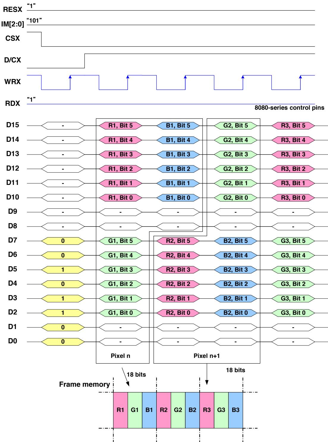
Note 1: The data order is as follows, MSB=D15, LSB=D0 and picture data is MSB=Bits 5, LSB=Bit 0 for Red, Green and Blue data.
