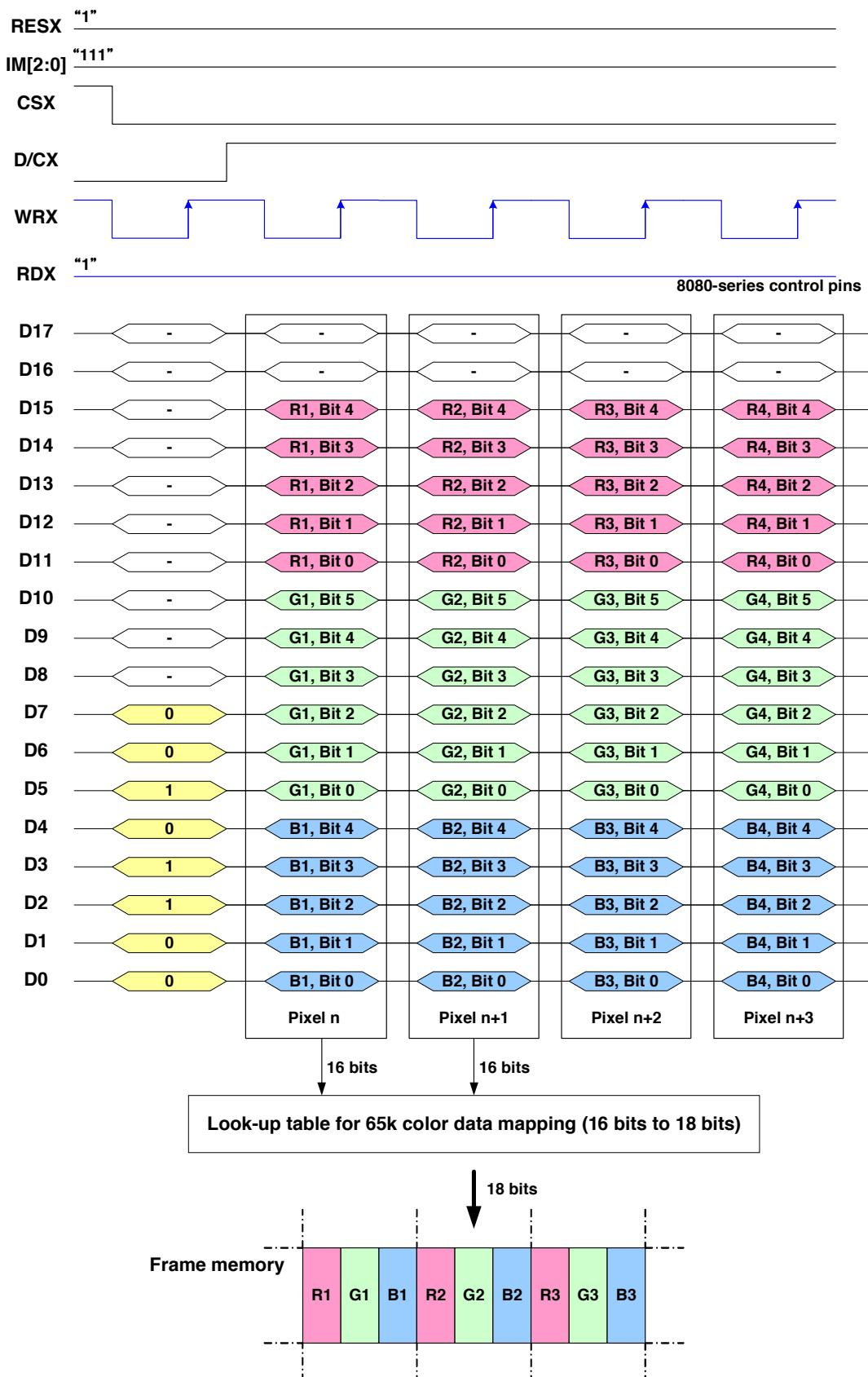
Note 1: The data order is as follows, MSB=D15, LSB=D0 and picture data is MSB=Bit 5, LSB=Bit 0 for Green, and MSB=Bit 4, LSB=Bit 0 for Red and Blue data.
