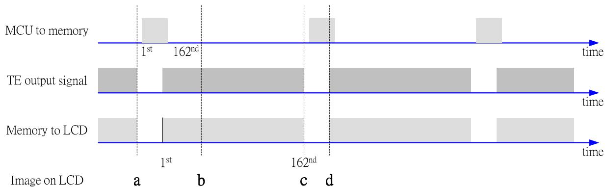
Data write to Frame Memory is now synchronized to the Panel Scan. It should be written during the vertical sync pulse of the Tearing Effect Output Line. This ensures that data is always written ahead of the panel scan and each Panel Frame refresh has a complete new image:
