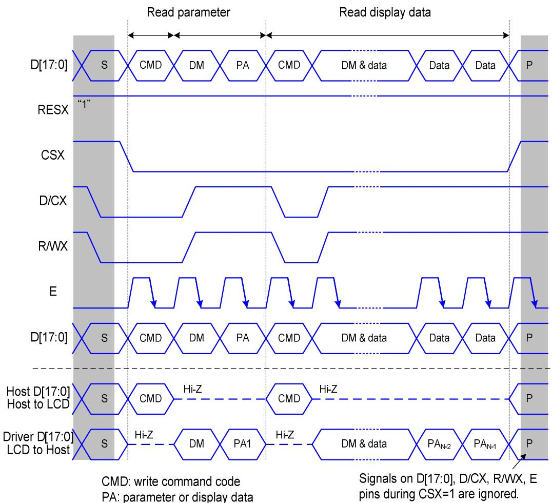
Figure 15 6800-series Parallel Bus Protocol, Read Data from Register or Display RAM
