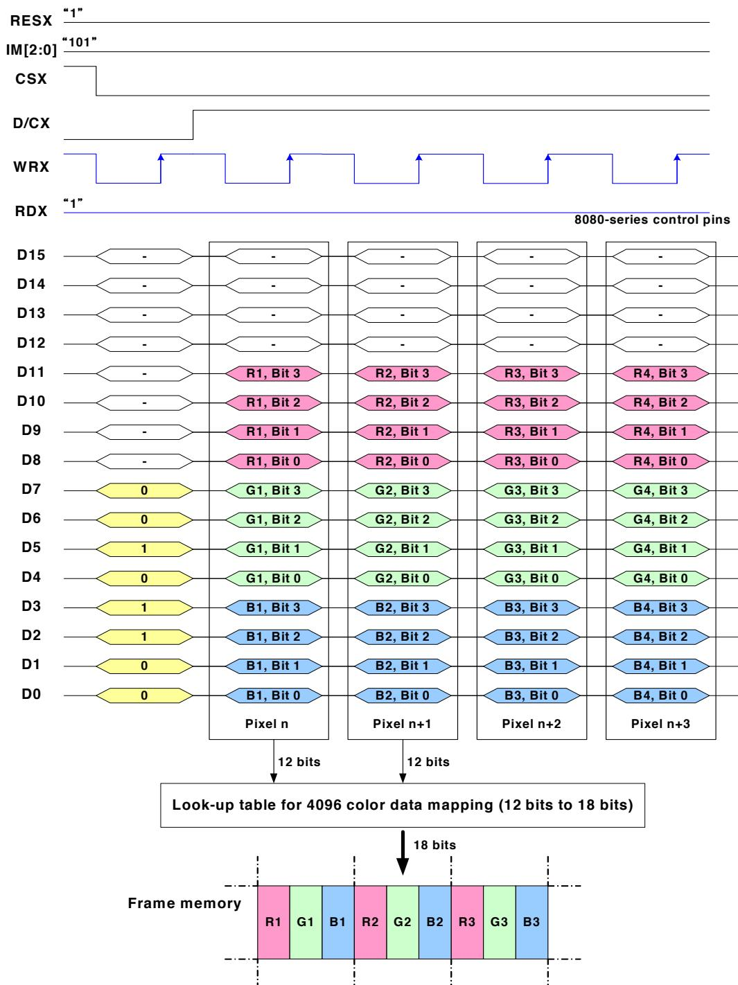
Note 1: The data order is as follows, MSB=D11, LSB=D0 and picture data is MSB=Bit 3, LSB=Bit 0 for Red, Green and Blue data.
