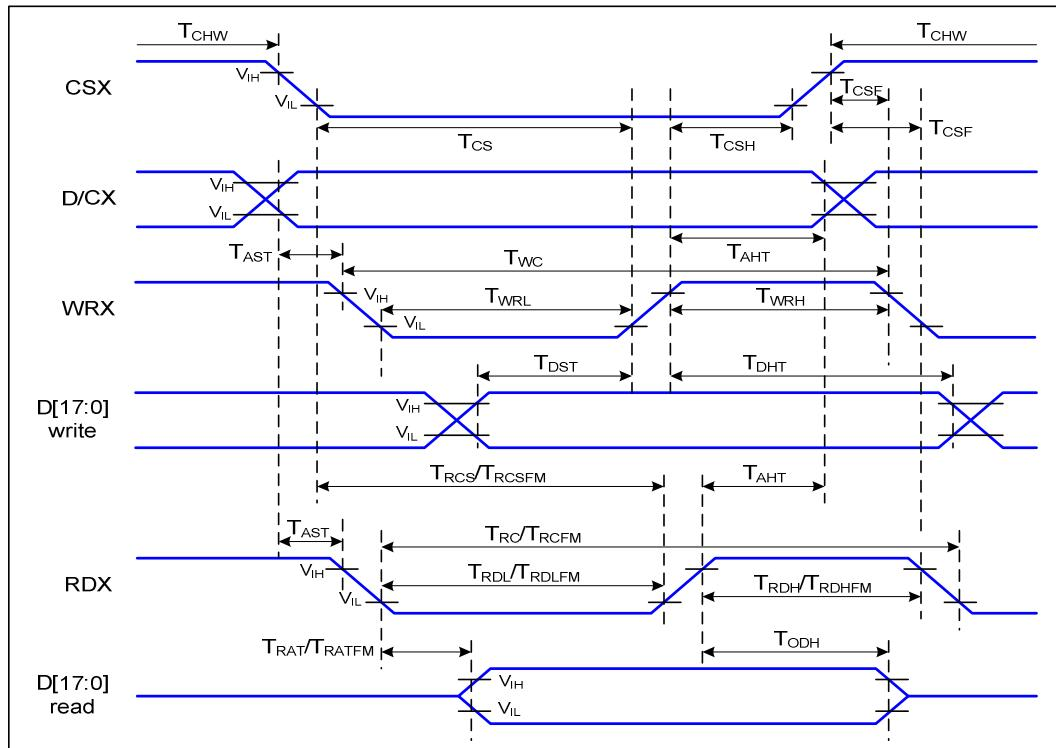
Figure 1 Parallel Interface Timing Characteristics (8080 Series MCU Interface)
