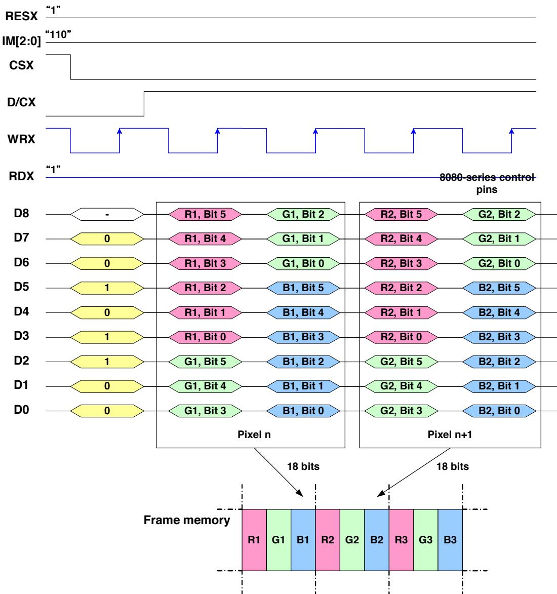
Note 1: The data order is as follows, MSB=D8, LSB=D0 and picture data is MSB=Bit 5, LSB=Bit 0 for Red, Green and Blue data.
