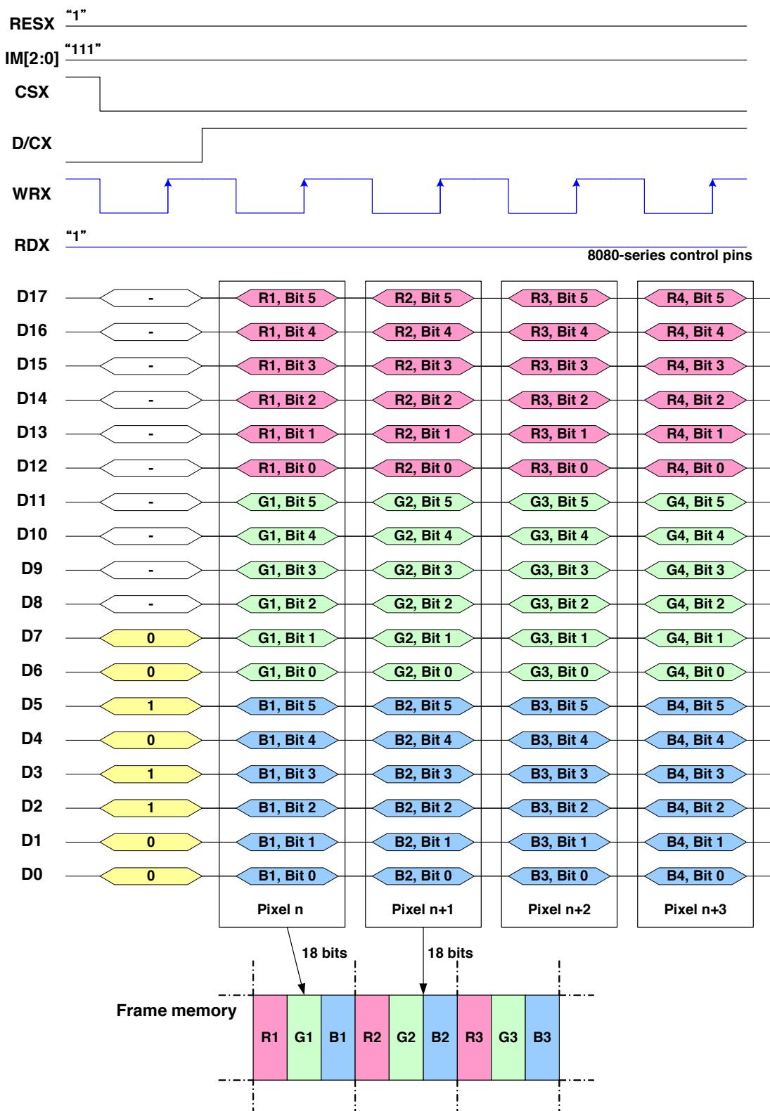
Note 1: The data order is as follows, MSB=D17, LSB=D0 and picture data is MSB=Bit 5, LSB=Bit 0 for Read, Green and Blue data.
